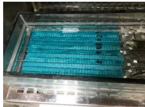
Fig. 6 PEN fiber/FRP specimens immersed in NaOH/NaCl solutions or water
