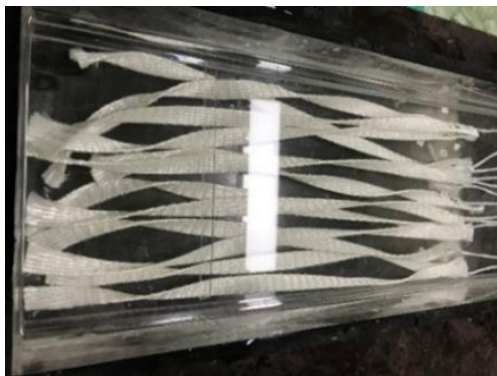
Fig. 6 PEN fiber/FRP specimens immersed in NaOH/NaCl solutions or water
